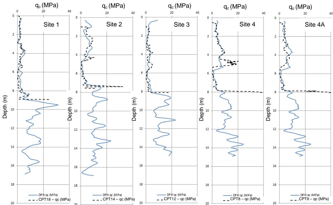
Figure 2: Halswell Sites 1 to 4 and 4A – comparison of CPT tip resistance and equivalent tip resistance derived from DPH data
