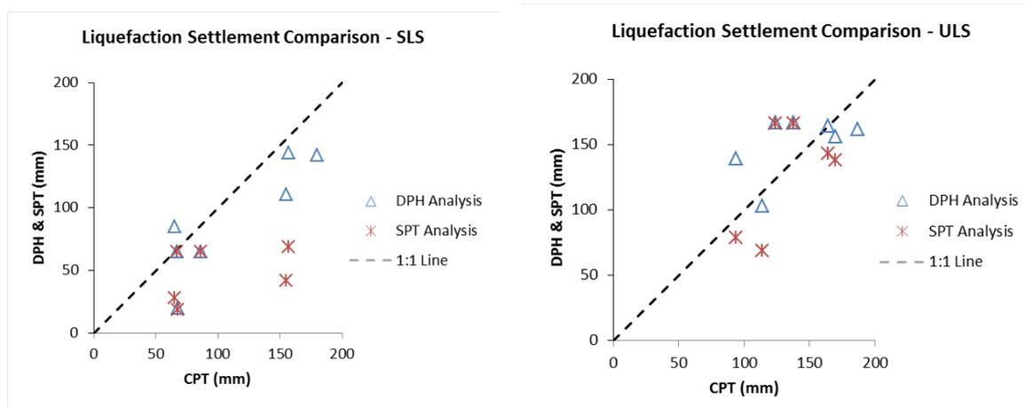
Figure 6: Settlement comparison (Test locations 1m to 2m apart)
