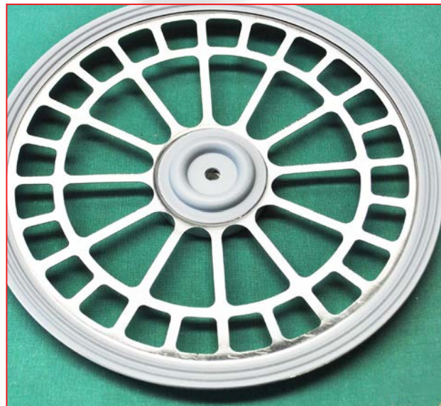
② Gluing of inner and outer ring onto the filter holder
