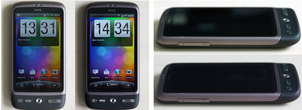
Fig. 3. HTC Desire smartphone before (left / top) and after (right / bottom) 640 disinfection cycles.
