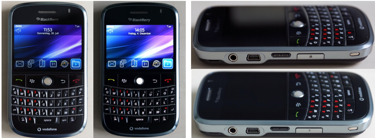
Fig. 6. BlackBerry Bold 9000 smartphone before (left / top) and after (right / bottom) 640 disinfection cycles.
