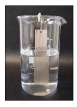
Standard test pieces (20 mm x 100 mm x 1 mm or 2 mm) with a total surface area of 0.00424 m² were 60% immersed in mikrozid® universal for 24 hours at a temperature of 35°C. The weight difference (increase/decrease) in  $g/m^2$  was determined and the test metals and disinfection solutions were subjected to visual examination.
