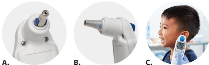
**A.** Inspect the probe lens for smudges or debris and clean with a dry lint free swab if needed. If lens does not easily clean, please see instruction manual for proper cleaning instructions.
