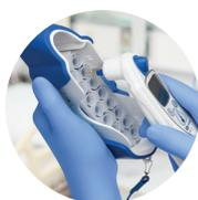
6 When loading probe covers into base unit, do not touch plastic film on the distal tip of the probe cover with your fingers.
