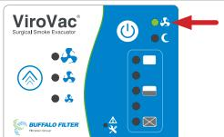
Press the Suction On / Standby Button on the membrane panel to illuminate the "suction on" green LED, indicating active suction.
