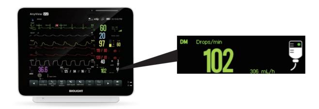
The DM module can monitor the drip rate all the time during the infusion. When the infusion is completed, the module will clamp up the infusion tube in order to avoid the blood reflux.
